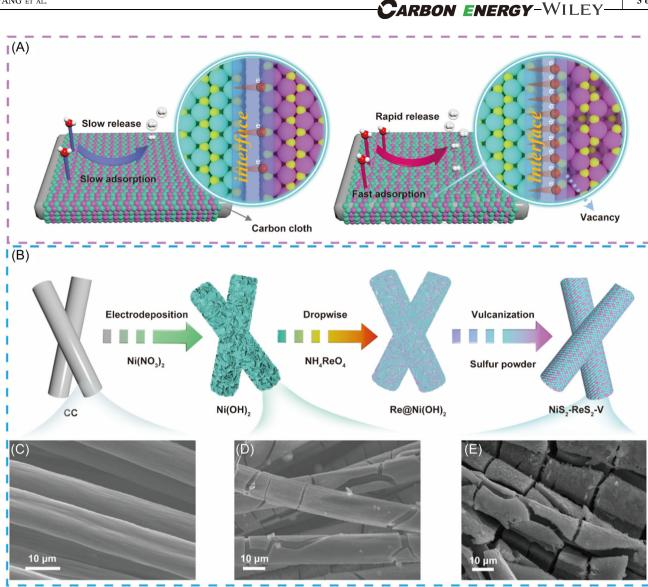
**FIGURE 1** (A) Schematic illustration of charge redistribution under the regulation of the BIEF. (B) Schematic illustration of the synthesis of NiS<sub>2</sub>-ReS<sub>2</sub>-V. SEM images of (C) carbon cloth (CC), (D) Ni(OH)<sub>2</sub>, and (E) NiS<sub>2</sub>-ReS<sub>2</sub>-V<sub>1</sub>.
