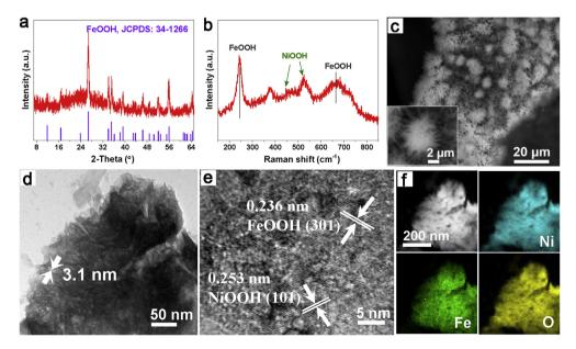
Fig. 1 — - (a) XRD pattern of collected powder. (b) Raman spectrum, (c) SEM image, (d) TEM image, (e) high-resolution TEM image, and (f) HAADF-STEM image and the corresponding elemental mappings of O, Ni and Fe from FeOOH–NiOOH/NF-24 h.
