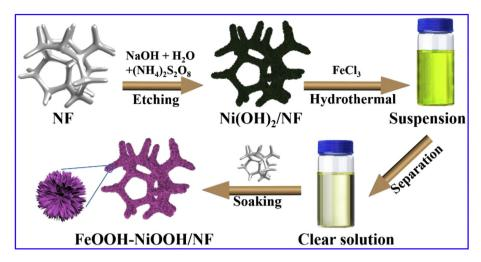
Scheme 1 - Schematic illustration of the synthesis process for FeOOH-NiOOH/NF.
