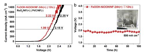
Fig. 4 – (a) Overall water splitting of different catalysts in two-electrode system. (b) Chronopotentiometric test of FeOOH–NiOOH/NF-24 h||-12 h catalysts at a fixed current density of 500 mA cm<sup>-2</sup> for 100 h (Inset: test photo).
