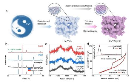
Figure 1. (a) Schematic illustration for synthesizing of Co/VN@NC. (b) XRD patterns and (c) Raman spectra of Co@NC, VN@NC, and Co/VN@NC, respectively. (d)  $N_2$  adsorption and desorption isotherms of Co/VN@NC (insert: the corresponding pore size distribution).
