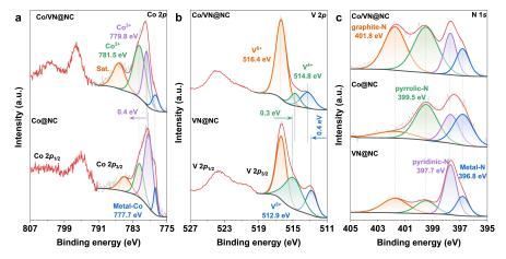
Figure 3. High-resolution X-ray photoelectron spectroscopy (XPS) spectra of (a) Co 2p, (b) V 2p, and (c) N 1s regions in Co/VN@NC, Co@NC, and VN@NC, respectively.
