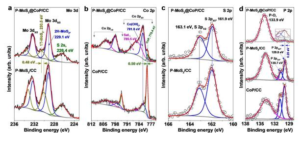
Figure 3. High-resolution XPS spectra of the a) Mo3d and b) Co2p and c) S2p and d) P2p regions of P-MoS2@CoP/CC, P-MoS2/CC, and CoP/CC, respectively.
