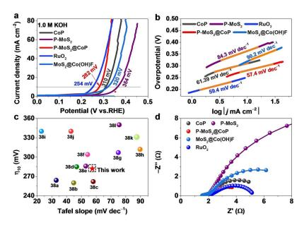
Figure 5. Electrocatalytic OER performance in 1.0 m KOH. a) LSV polarization curves and b) corresponding Tafel slopes of different catalysts. c) Overpotentials of recently reported catalysts at 10 mAcm<sup>-2</sup>; corresponding Tafel slopes are reported in Table S5. d) Nyquist plots of different catalyst.
