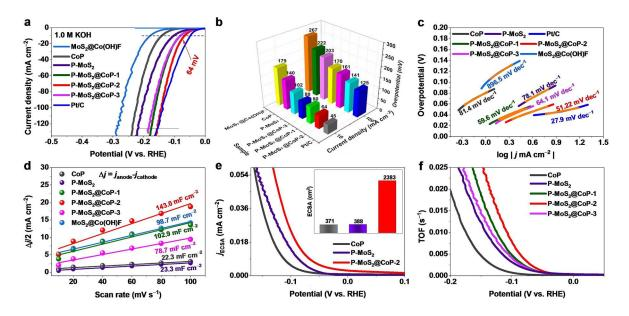
Figure 4. Electrocatalytic HER performance: a) LSV polarization curves, b) comparison of overpotentials at 10 and 100 mA cm $^{-2}$  for P-MoS $_2$ @CoP-2 and other references, c) corresponding Tafel slopes, d)  $C_{\rm el}$  of different catalysts in 1.0 m KOH. (e) ECSA-normalized LSV curves (Inset: a bar chart of the ECSA) of CoP, P-MoS $_2$ , and P-MoS $_2$ @CoP-2. f) Potential-dependent TOF curves of CoP, P-MoS $_2$ , P-MoS $_2$ @CoP-1, P-MoS $_2$ @CoP-2, and P-MoS $_2$ @CoP-3, respectively.
