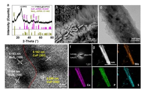
Figure 2. a) XRD patterns of P-MoS<sub>2</sub>@CoP/CC. b, c) SEM images of P-MoS<sub>2</sub>@CoP/CC. d) TEM image, e) HR-TEM image and f) SAED of P-MoS<sub>2</sub>@CoP/CC. g) HAADF-TEM image and corresponding elemental mappings of P-MoS<sub>2</sub>@CoP/CC (color online).
