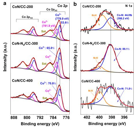
Fig. 4. XPS spectra of (a) Co 2p and (b) N 1 s regions from CoN/CC-200, CoN-N<sub>d</sub>/CC-300 and CoN/CC-400, respectively.
