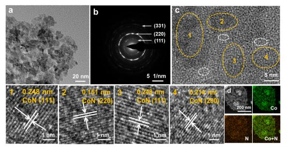
Fig. 3. (a) TEM image, (b) SAED and (c) High-Resolution TEM images, and (d) HAADF-STEM image and corresponding elemental mappings of CoN-N<sub>d</sub>/CC (color online).
