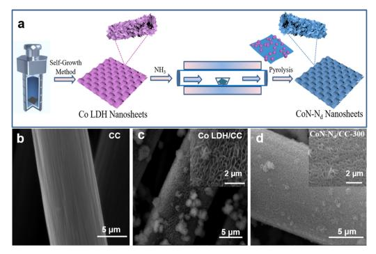
Fig. 1. (a) Schematic illustration of the synthesis of CoN-N<sub>d</sub>/CC. (b-d) SEM images of CC, Co LDH/CC, and CoN-N<sub>d</sub>/CC.
