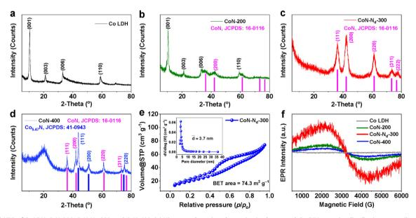
Fig. 2. (a-d) XRD of Co LDH, CoN-200, CoN-N<sub>d</sub>-300, and CoN-400. (e) Nitrogen adsorption–desorption isotherms and the BJH pore-size distribution curves (inset) of CoN-N<sub>d</sub>-300. (f) The ESR spectra of CoN-N<sub>d</sub>-300 (peeled off from the CC).
