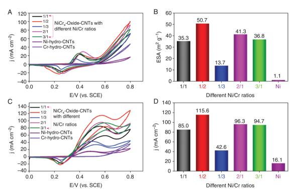
Fig. 4: (a) CV curves of NiCr<sub>x</sub>-oxide-CNTs with different Ni/Cr ratios, Ni-hydro-CNTs and Cr-hydro-CNTs in 1.0 M KOH. (b) The summarized ESA values from (a). (c) CV curves of different catalysts in 1.0 M KOH + 0.33 M urea. (d) The summarized forward current densities from (c).
