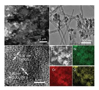
Fig. 2: (a) SEM, (b) TEM and (c) high-resolution TEM images of  $\rm NiCr_2$ -oxide-CNTs. (d) EDS mappings of  $\rm NiCr_2$ -oxide-CNTs with Ni, Cr and O elements
