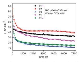
Fig. 5: Chronoamperometric curves of  $\rm NiCr_x$ -oxide-CNTs catalysts with different Ni/Cr ratios at a constant potential of 0.45 V (vs. SCE) in 1.0 M KOH + 0.33 M urea for keeping 7200 s
