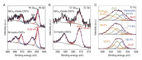
Fig. 3: High-resolution XPS regions of (a) Ni 2p, (b) Cr 2p and (c) O 1s from NiCr<sub>2</sub>-oxide-CNTs, Ni-hydro-CNTs and Cr-hydro-CNTs
