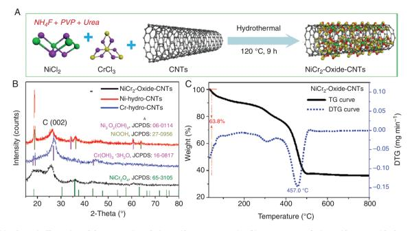
Fig. 1: (a) Schematic illustration of the preparation of NiCr<sub>2</sub>-oxide-CNTs composite. (b) XRD patterns of NiCr<sub>2</sub>-oxide-CNTs, Ni-hydro-CNTs and Cr-hydro-CNTs. (c) Thermogravimetric (TG) and differential thermogravimetric (DTG) curves of NiCr<sub>2</sub>-oxide-CNTs with a heating rate of 2.5°C min<sup>-1</sup> under O<sub>2</sub> atmosphere.
